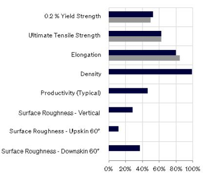
Bar plot is generated by normalizing typical material data (containing both horizontal and vertical data) against a range defined for each material family. For nickel-based alloys, the ranges are as follows: 0.2%YS: 0-1200 MPa, UTS: 0-1500 MPa, Elongation: 0-50%, Density: 99-100%, Productivity: 5-60 cm³/h, Surface Quality (all): 5-40 µm. 0% in the bar plot indicates the lower range value, 100% indicates the upper range value.
