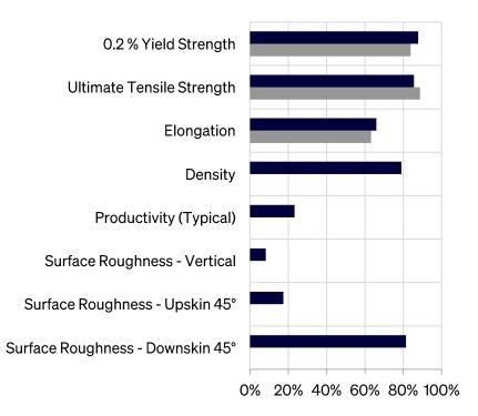
Bar plot is generated by normalizing typical material data (containing both horizontal and vertical data) against a range defined for each material family. For steel-based alloys, the ranges are as follows: 0.2%YS: 0-600 MPa UTS: 0-750 MPa, Elongation: 0-60%, Density: 99-100%, Productivity: 5-60 cm³/h, Surface Quality (all): 5-40 µm. 0% in the bar plot indicates the lower range value, 100% indicates the upper range value.
