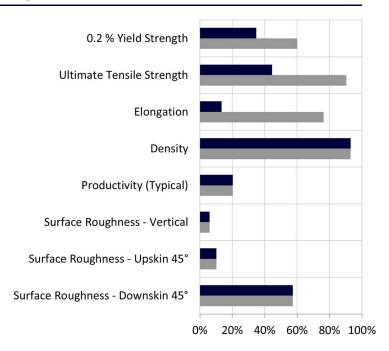
Bar plot is generated by normalizing typical material data (containing both horizontal and vertical data) against a range defined for each material family. For cobalt-based alloys, the ranges are as follows: 0.2%YS: 0-1150 MPa UTS: 0-1450 MPa, Elongation: 0-60%, Density: 99-100%, Productivity: 5-60 cm³/h, Surface Quality (all): 5-40  $\mu$ m. 0% in the bar plot indicates the lower range value, 100% indicates the upper range value.
