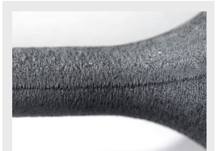
Figure 1: Good stitching: 150-micron misalignment between lasers, special contour countermeasures. Source: Colibrium Additive
